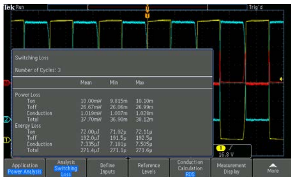
Figure 31: Switching Loss measurements.
