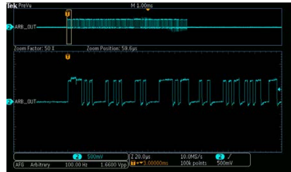
Figure 21: Noise-free CAN signal generated by the ARB.
