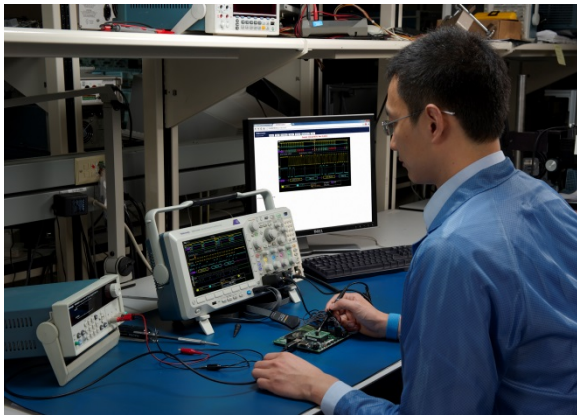
Figure 7: Decoding an I 2 C bus, while viewing waveforms.
