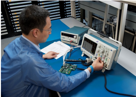
Figure 24: MDO3000 with differential voltage probe and current probe.
